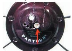
**STEP 2.** The hub allows adjustment for different types of fork drop-outs and travel trajectories. For Dahon aluminum forks and bikes, the trajectory adjustment screw should be set to position hole #1 (to the front of the bike). Be sure not to use the other holes as using the incorrect trajectory could result in damage to the bike or serious injury or death to the rider.
