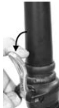
**E:** **step 2c:** Loosen the two adjuster bolts and align the stem and handlebar with the handle post as pictured.
