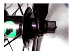
**STEP 3.** Make sure that the wheel is properly positioned in the fork. The trajectory adjustment screw must sit in the rear most position of the fork drop-out. Note that the small silver screws in the picture (above right) should be pointing forwards and downwards. That's it – now have fun riding!
