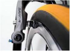
**STEP 1.** Adjust the front brake pads so that they are aligned with the uppermost portion of the brake track on the rim. Spin the wheels to make sure that the brake pads do not contact the tire at any point.
