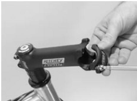
**E:** Remove the screws from the stem face plate.
