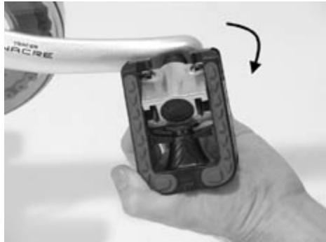
**E:** If you have folding pedals, you can fold them by pushing the pedal body inwards and flipping the pedal body downwards.
