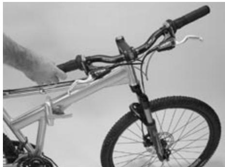
**E:** To fold your bicycle, simply reverse the steps described on pages 9-26. Tip: For a faster fold on an XA model, there is no need to remove the handlebar - simply loosen the stem and star nut bolts and twist the stem and handlebar 90 degrees to the right. Fold the frame as usual.
