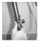
**STEP 8b:** Rotate the stopper hook so that it secures the post latch.
