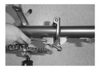
STEP 9: Open the frame latch lever.
