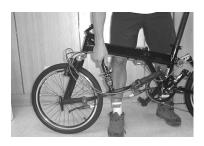
**STEP 9:** Swing the handlepost into the folded position: upside down and flush against the front wheel and frame.
