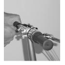
**STEP 8c:** Open the handlepost stem quick release latch and rotate the handlebar forward until it stops.
