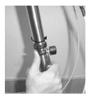
**STEP 7c:** Push the handlepost latch inwards until it snaps closed. Rotate the stopper hook so that it secures the post.
