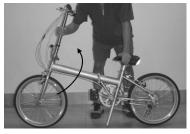
**STEP 6:** Swing the handlepost up to its vertical position.
