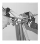
STEP 2c: Undo the handlepost stem quick release latch and rotate the handlebar so the brake levers are pointed straight up.
