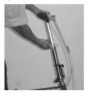
**STEP 9b:** Adjust the Telescope™ stem to the desired height.
