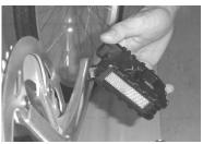
**STEP 11B:** If you are unfolding your pedals, flip the pedal into the horizontal position. Be careful not to pinch your fingers.
