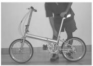
**STEP 10:** Open the seatpost quick release lever and raise the saddle to the desired height. Close the seatpost quick release lever. Be sure not to raise the seatpost beyond the safety line marked on the seatpost.
