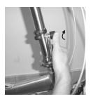
**STEP 7b:** Push the handlepost latch inwards until it snaps closed.
