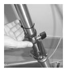
**STEP 3b:** Rotate the stopper hook away from the handlepost latch.
