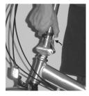
**STEP 7a:** Push the handlepost latch inwards until it snaps closed.
