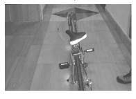
**STEP 6**: Open the seat post quick release. Lower the seat post. Twist the saddle 45 degrees to the left. Close the quick release.
