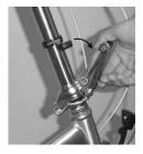
**STEP 4b:** Unlock the handlepost latch by pulling it away from the handlepost.
