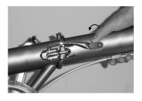
**STEP 5:** Move the frame latch safety hook into the closed position.
