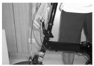
**STEP 8:** Pull outwards to open the handlepost latch.
