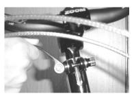
**STEP 2:** Open the quick release on the Telescope handle post.
