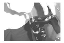
STEP 1: Loosen the stem steerer bolt.
