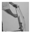
**STEP 2b:** Move the stem into the folded position.
