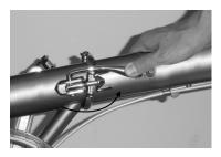
**STEP 4:** Lock the frame latch lever by pushing it in towards the frame. It should require 6 kg. of force to close.
