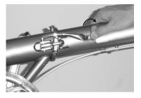
**STEP 8:** Move the frame latch safety hook to the open position.
