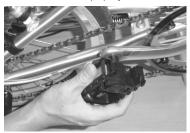
**STEP 12:** Snap the folding pedal(s) into the folded position by pushing the pedal body inwards and rotating downwards.
