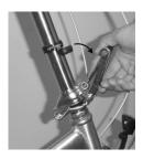
**STEP 4c:** Rotate the stopper hook away from the handlepost latch. Unlock the handlepost latch by pulling it away from the handlepost.
