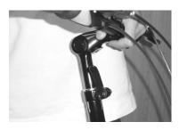
**STEP 3:** Move the MicroAdjust stem up or down to the desired height.
