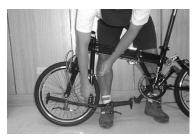
**STEP 10:** Open the handlepost quick release and pull out the stem so that the handlebars clear the bottom of the fork.
