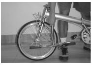
**STEP 5:** Swing the handlepost into the folded position: upside down and flush against the front wheel. Be sure the front wheel stays parallel to the frame. When folded properly, the handlebars should sit just below the wheel axle.
