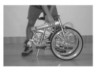
**STEP 10:** Fold the frame in half by swinging the front half of the frame back until the two wheels are parallel.
