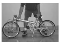
**STEP 2:** Unfold the frame by swinging the front and rear halves of the frame apart.
