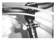
**STEP 2:** Open the quick release on the Telescope stem.
