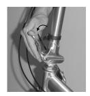
**STEP 4a:** Unlock the handlepost latch by pulling it away from the handlepost.
