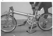
**STEP 7:** Rotate the cranks so that the left crank is pointed straight forward.
